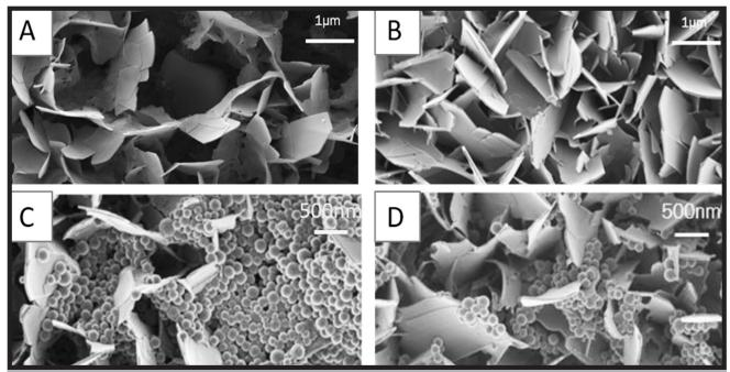
FIG. 5. SEM microphotographs of the bioactive layer on the ZrO<sub>2</sub> substrate after the first (A) and the second (B) step of the coating process and NPs deposited on the ZrO<sub>2</sub> substrates by drop-sitting method (C) and during the CaP layer preparation process (D).
