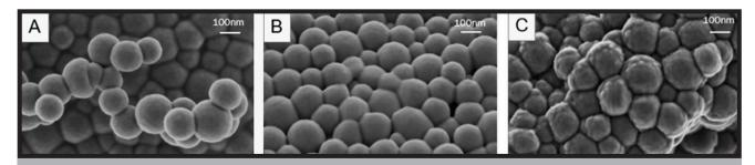
FIG. 2. SEM images of different types of nanoparticles: A – empty nanoparticles (PLGA); B – nanoparticles loaded with gentamicin (PLGA\_Gent); C – nanoparticles loaded with bacitracin (PLGA\_Bct).
